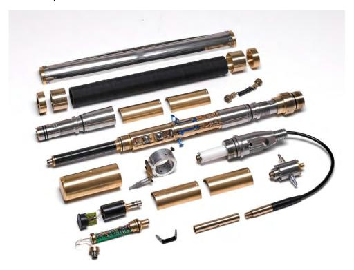
Figure 1.1 The 95mm High Pressure Dilatometer
